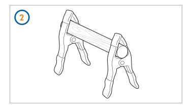
Attach a spring clamp to either end of the rod.
