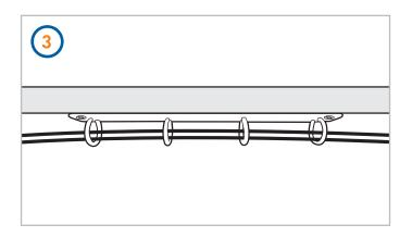
You can now use the binder to keep cables neat and out of harms way. Being able to open and close the binder makes it easy to add and remove cables as you wish.
