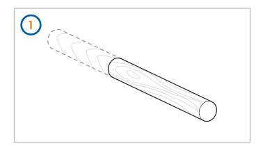
Cut the wooden rod to size according to how wide you require the sawhorse.
