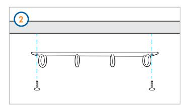
Screw through the holes left by the rivets and into the underside of the desk.
