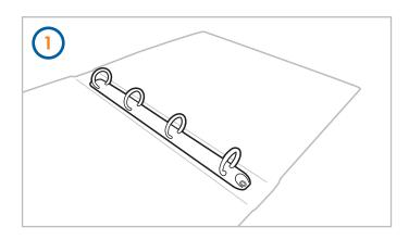
Use a knife to cut the metal ring binder away from the cardboard folder. When you have separated the metal binder from the folder use a pair of pliers to remove the rivets at either end.
